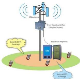
Gambar 1 BTS ( Base Transceiver Station )
