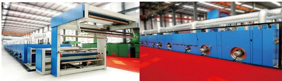
**Gambar 1 Mesin *Stenter Finishing***
