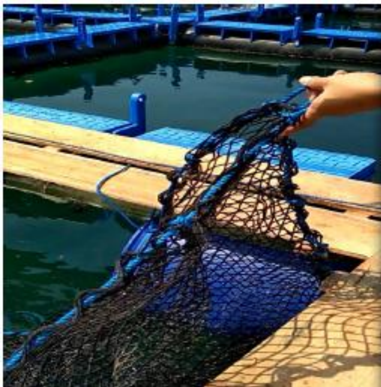
Gambar Z6 Model sambungan antar jaring
